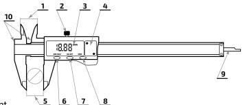
Switch digital measurement on by moving the jaw or using the power button. Set the jaws to minimal value and calibrate a zero value on the display using the button "Zero". Perform your measurement and read the results off the display.
