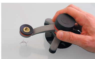
2. the RETECH tool holder is fixed above the damaged spot, ...
