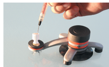
3. the injection cylinder is screwed in and filled with RETECH filling resin, ...
